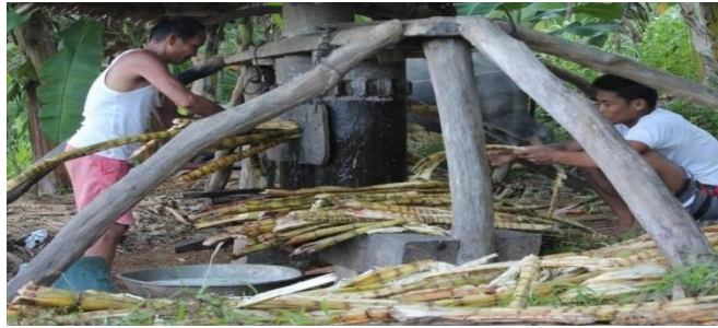
Fig. 5. Extraction of basi with wherein 5 pieces of sugarcane inserted into the “trapitsihan”.
