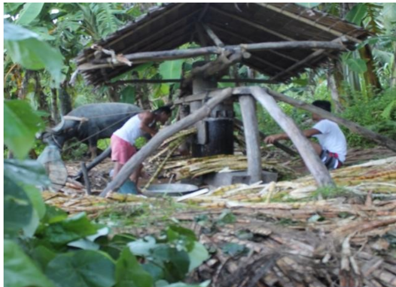
Fig. 6. Extraction of the basi, with the carabao used to twirl around the trapitsihan to undergo the production process. Manual operation can also be done.
